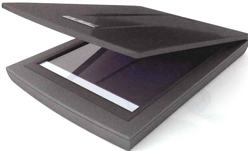
Figure 5.08 A flatbed scanner scans a document automatically
