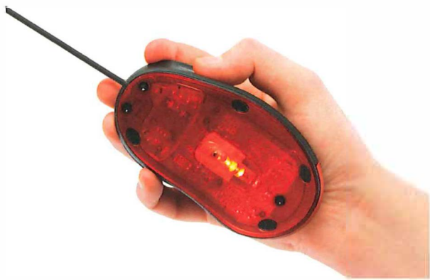
Figure 5.05 This newer style of mouse uses an optical laser to move the pointer
