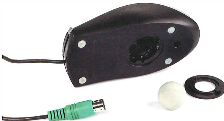
Figure 5.04 This older style of mouse uses a roller ball to move the pointer
